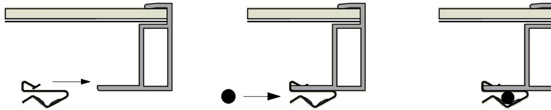
Mounting cable clamp on insert profile.
