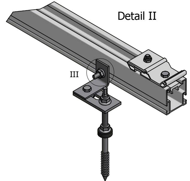
The groove of the bolt corresponds with the orientation of the bolt head.
